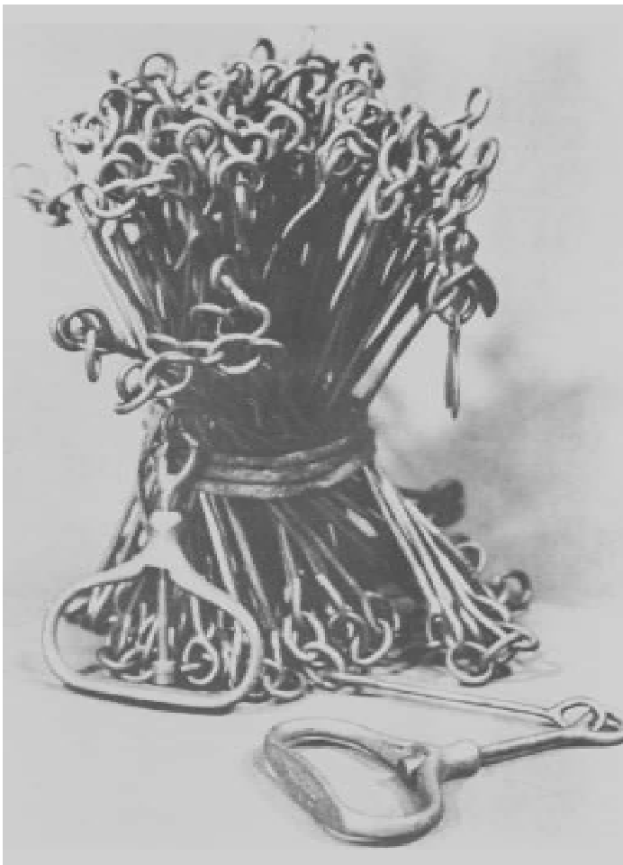
Picture of Gunther's half-chain, the type used by Mason and Dixon. From The Mason and Dixon Line: Story for a Bicentennary 1763-1963 .
